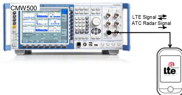
Figure 4-4: CMW500 with advanced RF frontend and DUT
